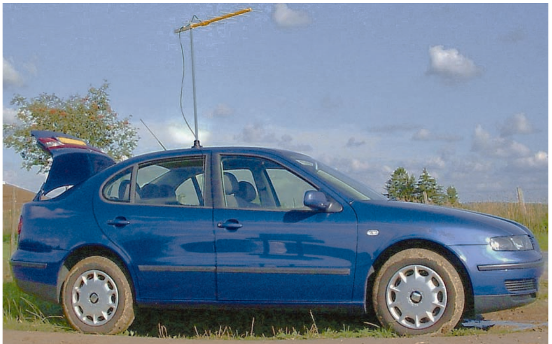
● David Butler says that the WA5VJB design antenna for 432MHz is a very effective beam antenna that will fit easily in the boot of a smaller car.
